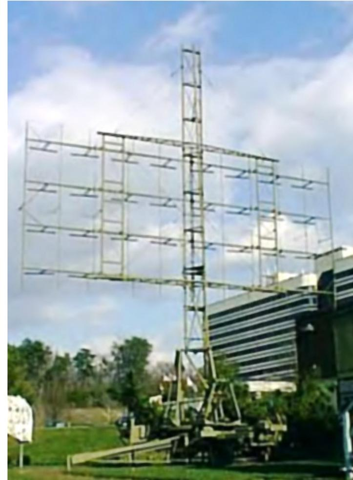
SCR-270-B radar antenna
