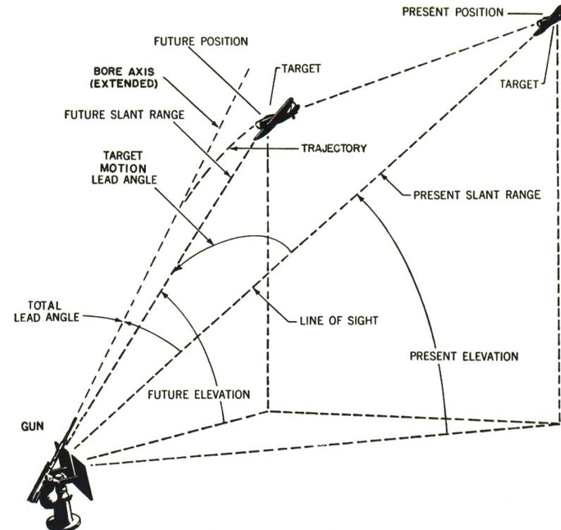
FIGURE 26A1.—Fire control problem; lead angle.
