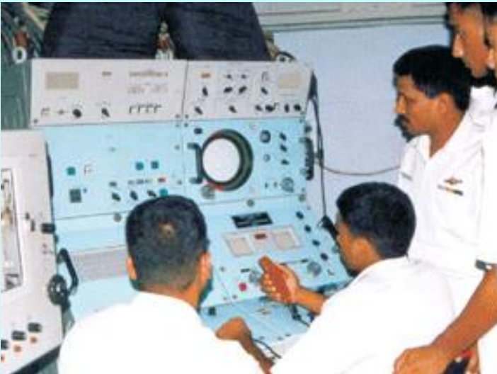
MGK-400 operator console
