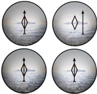
VIEWS SEEN BY EYES BEFORE COMPENSATOR WEDGES ARE ADJUSTED
